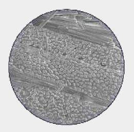
**Figure 5:** Oriented fiber layers as seen in a SEM image of an implant cross-section<sup>a</sup>
