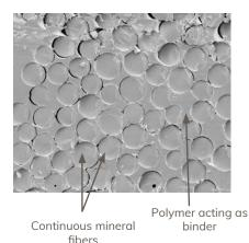
Figure 3: Scanning Electron Microscope (SEM) cross-section of OSSIO*fiber*, highlighting both material components.<sup>a</sup>
